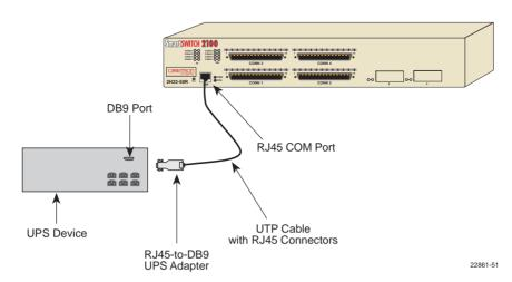
Figure 5-2 Uninterruptible Power Supply (UPS) Connection
